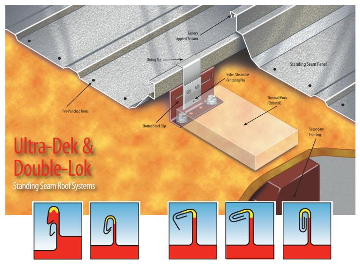
Ultra-Dek<sup>®</sup> Seamed with an interlocking snap seam making installation faster and easier.
